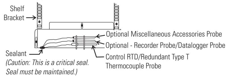
**Figure 1-3.** Chamber Probe(s)
