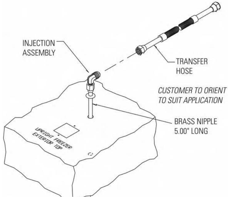
**Figure 5-1.** Injection Assembly
